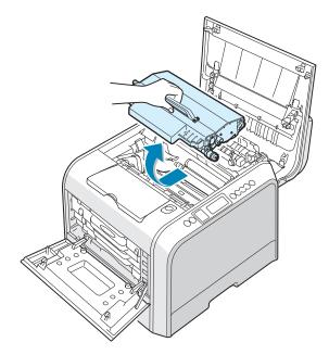
6 Lift the handle of the used imaging unit and use it to pull the imaging unit out of the printer.
